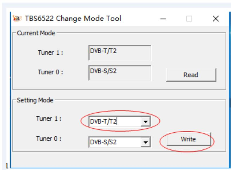
4) Remember to connect the corresponding antenna after you set a new mode.
